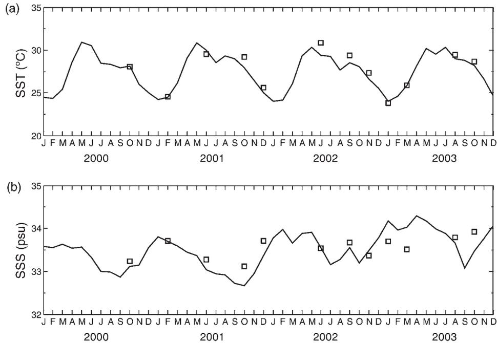
**Figure 3.** Comparison of modelled (a) sea surface temperature (SST) and (b) sea surface salinity (SSS), with the SEATS observational data from 2000 to 2003. Lines are model predictions, open squares are observations.
